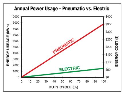
Comparing Traditional and Integrated Rod-style Linear Actuators: How to choose the best solution for motion control applications 9900-9196\_01
